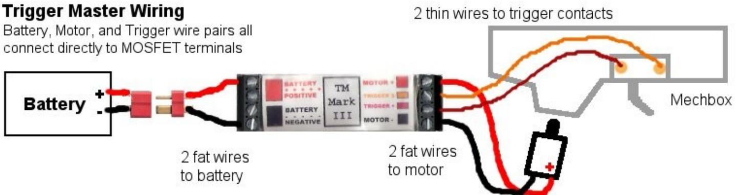
**NOTE:** There are two "Battery +" and two "Battery -" terminals on the Trigger Master. You need only connect the battery wires to one positive and one negative. (You do not need to use both "+" and both "-" terminals.)
