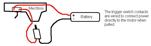
This is how the **Trigger Master** must be wired:
